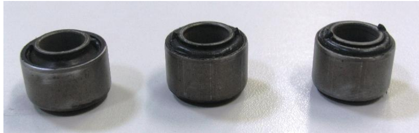
Şekil 2.8 Test Numuneleri (a. \varnothing 27\text{mm} b. \varnothing 26\text{mm} c. \varnothing 25,6\text{mm} )
