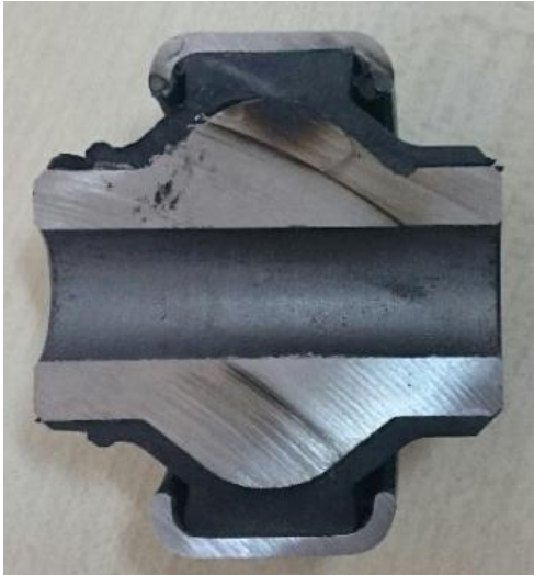
Figure 13: Picture of the new design after 1,1 million cycles of durability test.
