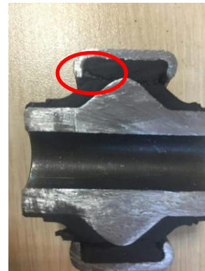
Figure 3: Cross-section of failed part.
